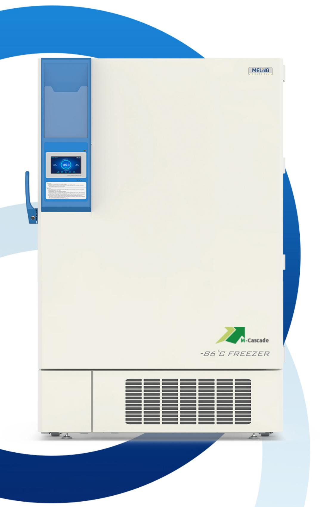
M-Cascade system ULT freezer that consists of two stages cascade cooling technology with absolute hydrocarbon refrigerant, which are R290 and R170 as natural gas. The inverter compressors programmed to help energy savings under long period preservation or provide fast temperature recovery while frequently door open to maintain specimens liveness.
